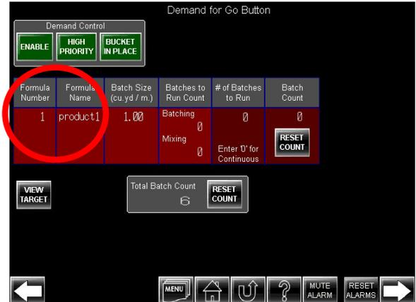
**NOTE:** *Concrete formulas are normally stored as one cubic yard or cubic metre, which is equal to 100% or 1.00. To batch a 2 cu. yd. or cu. m. mix, enter 2.00. To batch a 3/4 cu. yd. (cu. m.) mix, enter .75.*
