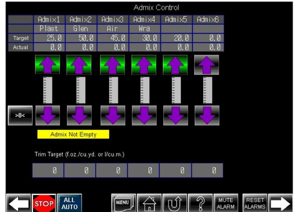
For Admix the top two rows display the Admix name and type. The following two rows display target and actual value amounts.
