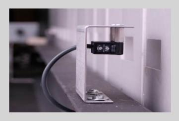
Last Bag Detector: a photo-sensor warns when only one bag remains, giving you enough warning to refill the dispenser. It reliably detects even small plastic bags.
