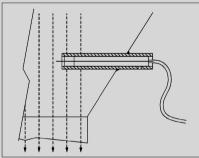
To monitor correctly and with fast response, the sensing cap needs to be in the flow region where material is drawn from the vessel.
