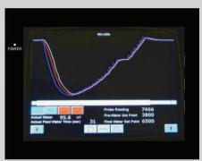
AquaControl's touch screen displays the moisture as mixing proceeds, allowing you to see the whole mixing process at a glance. Screen buttons override automatic operations, allowing you to pause or finish the process yourself if necessary.
