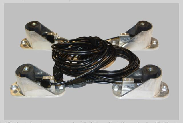
The Mini-Mount allows direct mounting of a platter in low profile platform scales. Four Mini-Mounts are located at the corners of a platform scale that can be any size and shape. Different capacities allow a single set of components to be used in a family of platform scales of many sizes and capacities. The Mini-Mount has overload protection built-in and can be used with confidence in applications where dropped items and other abuse is present.
