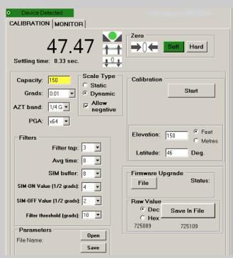
calibration and the second is applied during use. This system allows scales to be calibrated at one latitude and altitude and used at any other after the new coordinates are entered. The correction is within 0.01% anywhere on the earth's surface.
