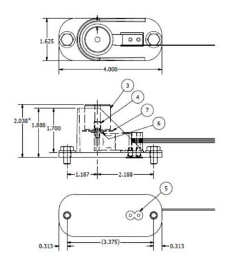
\* Overall height reduces to 1.89" at 130% of capacity
