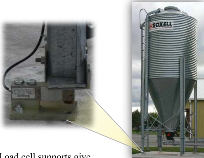
Load cell supports give highest accuracy
