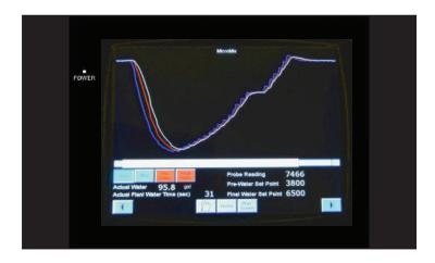
AquaControl's touch screen displays the moisture as mixing proceeds, allowing you to see the whole mixing process at a glance. Screen buttons override automatic operations, allowing you to pause or finish the process yourself if necessary.
